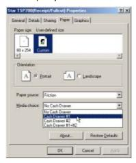
If you need to control the point at which the cash drawer is opened then you can use the 'control' font which is built into our drivers. Switch to the 'control' font and print a character 'A' to open cash drawer 1.
